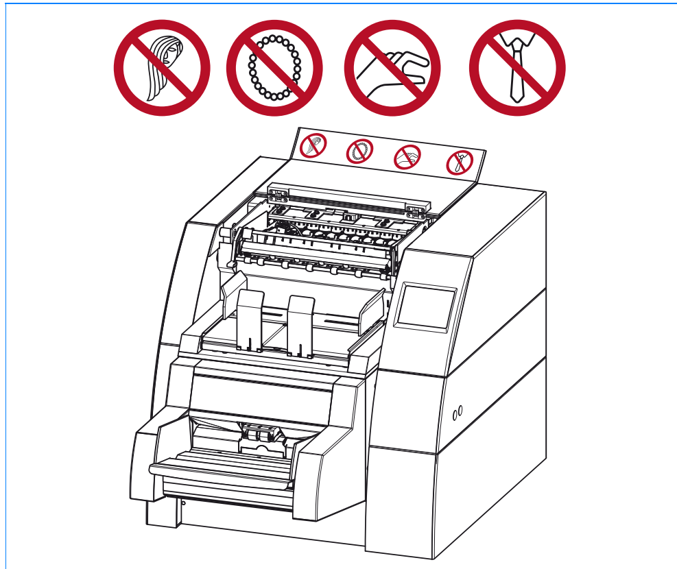
Fig. 3-3 Safety signs and labels at the upper outlet
